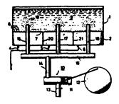
A fluidized bed furnace having a vessel with cooled or insulated walls and an inflow plate. A fluidized bed of inert material is maintained by air nozzles in the inflow plate and heated to the ignition temperature of coal. Pressure pipes deliver the coal and, if appropriate, additives such as lime, into the vessel below the upper boundary of the fluidized bed for combustion.
